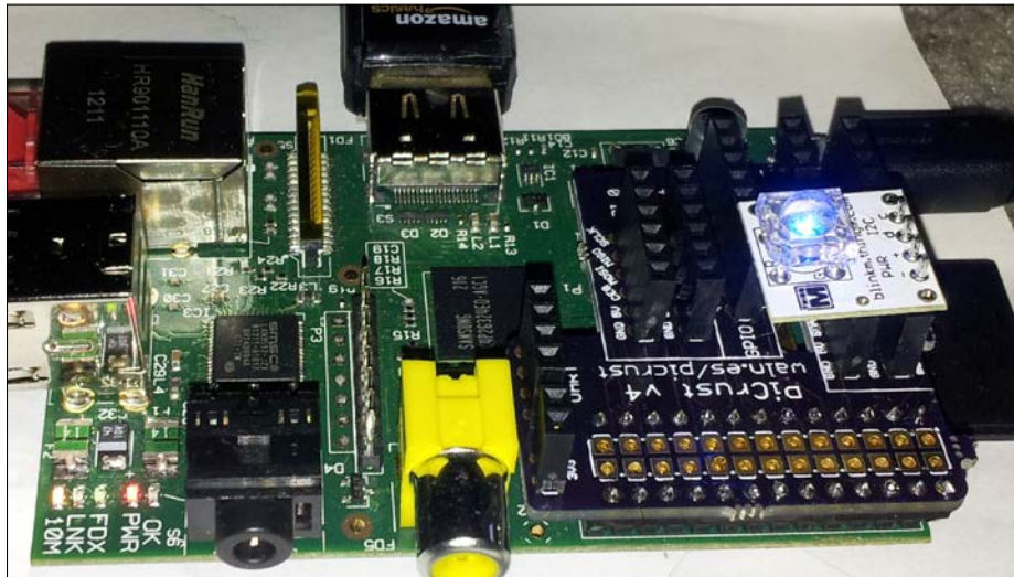
Pi Crust stacked on top of the Raspberry Pi
